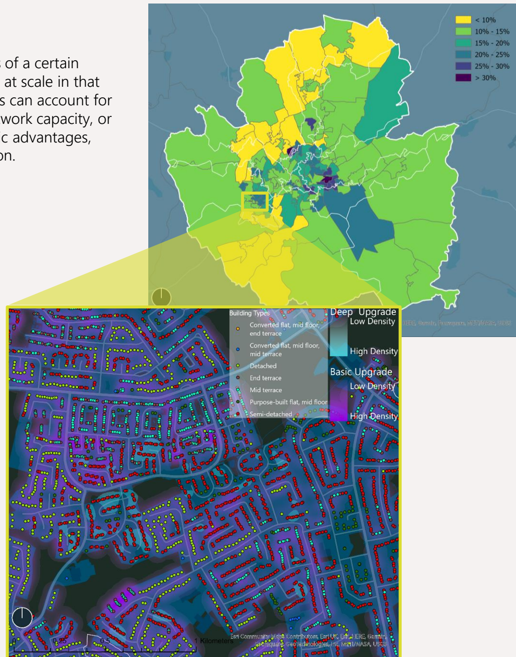
An example area of dwellings in the Acomb to Rufforth zone suitable for upgrades
